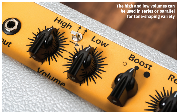
The line-out enables you to use the spring reverb as an independent effect
